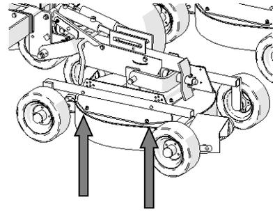
On the pivoting arm side remove the two axle stop pins and the center pivot bolt. Reposition the axle to the proper hole for the desired cutting height. Retighten the center pivoting bolt properly.
