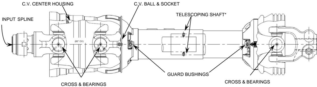
\* Inner & outer guards must be rotated to align holes for accessing telescoping shaft grease fitting.
