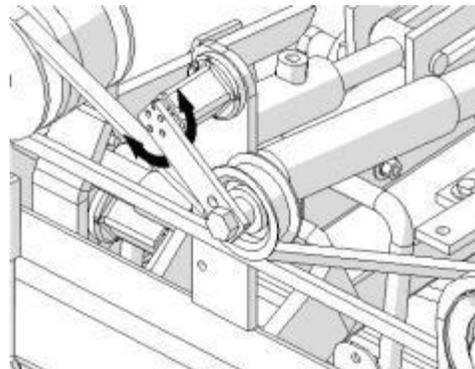
A tool is provided to allow easy release of belt tension using a 1/2” drive breaker bar or ratchet.
